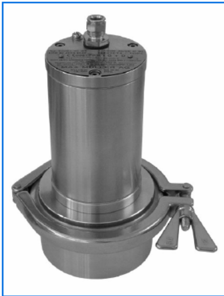
Sightglass light fitting, type EdelEx STERI-LINE 20 dH, 24 V, 20 W, EEx d IIC T4, Ex II 2 G + D, on metal fused sightglass, DN 100
